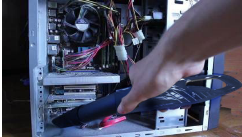
Fig 5.1.2 Gently clean the CPU with a vacuum cleaner
